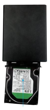
5. Place the front panel back on by placing it over the drive bay, and sliding it into place.
